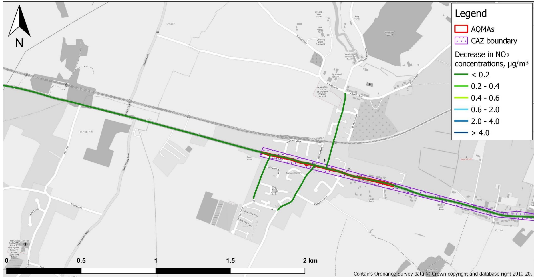
Figure 4-24 – The reduction in NO 2 concentrations around Newington for the pinch point option
