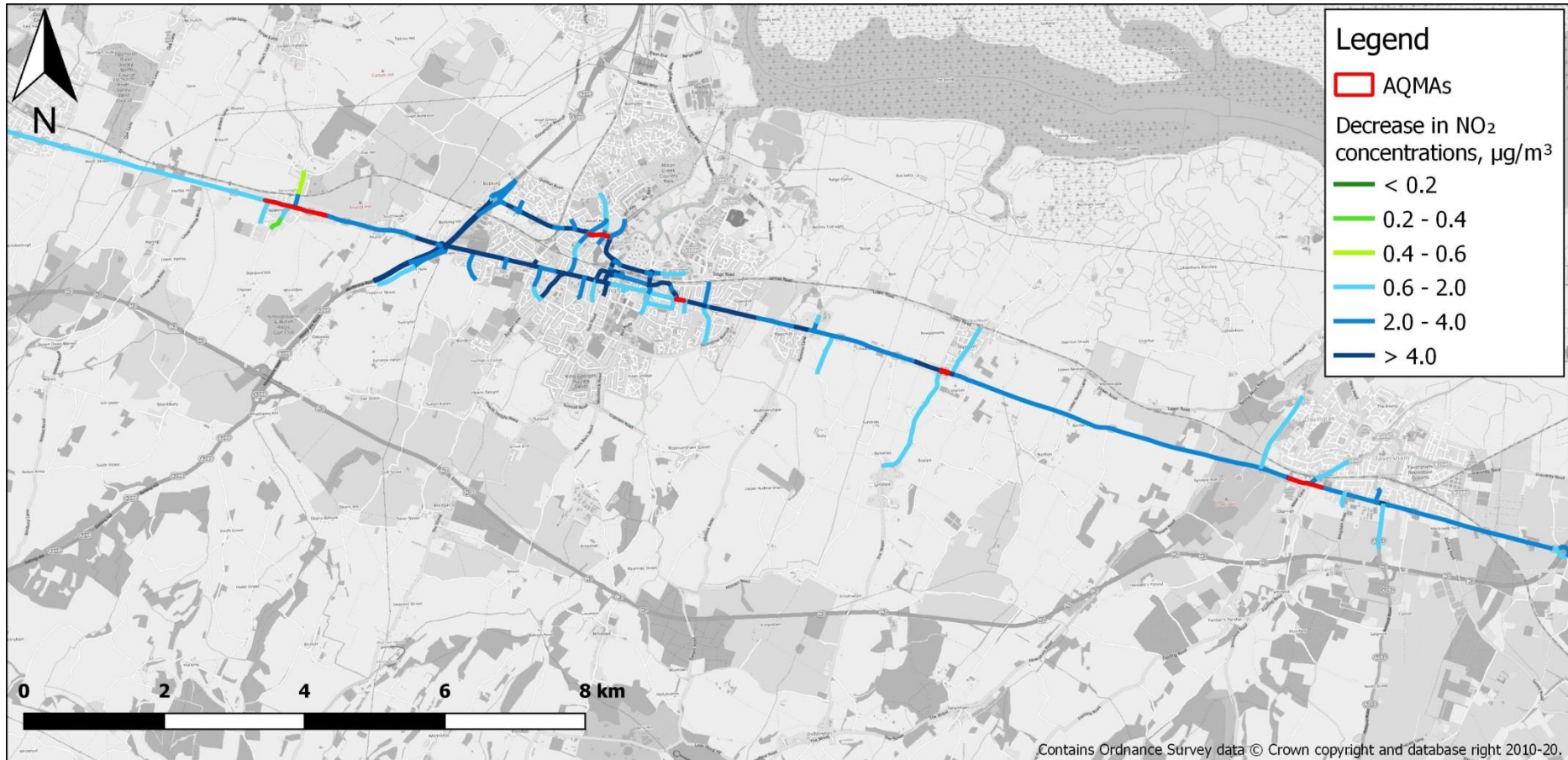
Figure 4-6 – The reduction in NO 2 concentrations along the A2 for the CAZ D option
