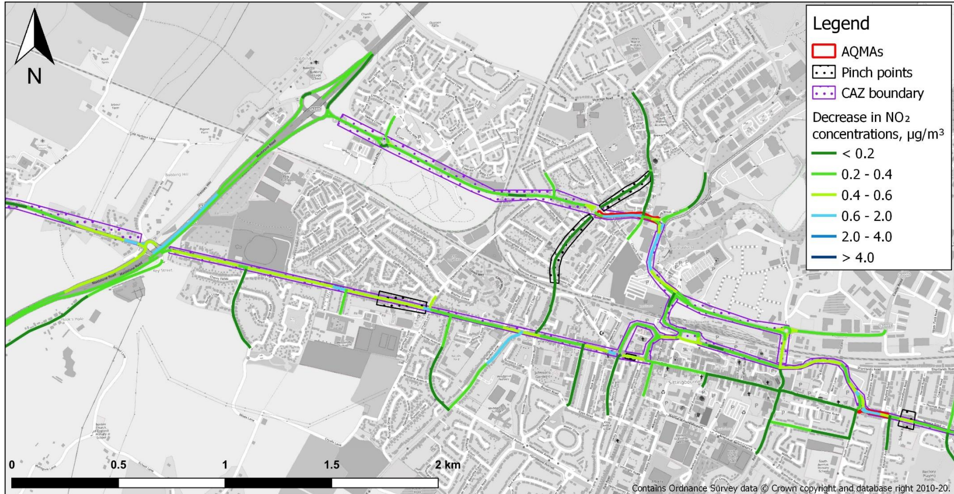
Figure 4-5 – The reduction in NO 2 concentrations around Sittingbourne for the CAZ B option
